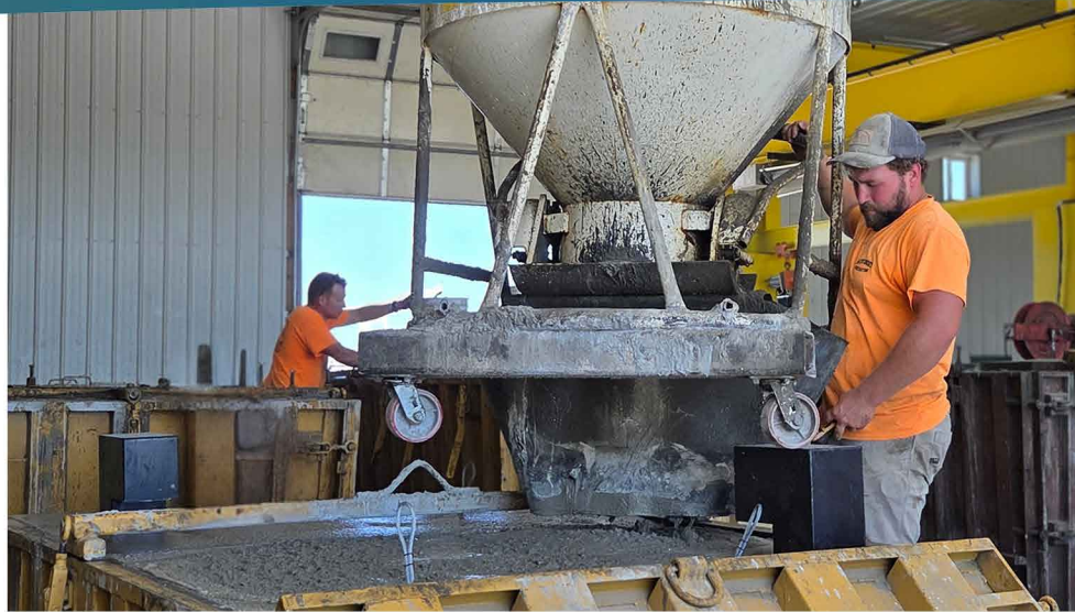
Lucas pours concrete into the rebar shell that will form a storm shelter, while his brother Tommy works on finishing a septic tank in the background.
